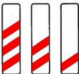
Countdown markers to a level crossing. Each line represents 1/3 of the distance to the crossing
