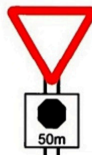
Distance to 'STOP' line ahead
